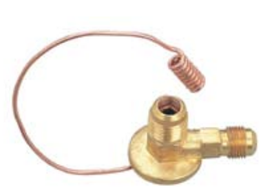
■ ■ CH-342 Can Tap Valve Forged brass body, strong and no leaking. Specially for R134A can 1/2" ACME female X 1/2" ACME male.
