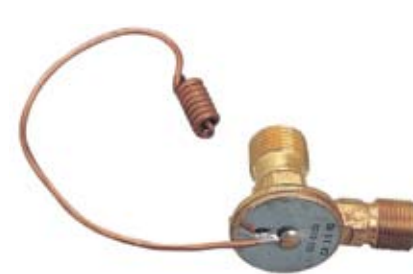
■ ■ CH-341 Line Piercing Valve Fits 3/16" thru 3/8" O.D. and has 1/4" flare connection for charging hose.
