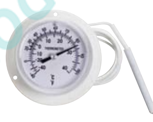
300RF22011 3" THERMOMETER WITH INTERGRATED SPRING CLIPS+ADAPTER HOUSING FOR 3 POSSIBILITIES TO MOUNT \phi 80mm CASE : ABS WHITE, BACK ADJUSTMENT RANGE : -40~-40°C , -40~100°C
