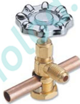
■ ■ CH-341 Line Piercing Valve Fits 3/16" thru 3/8" O.D. and has 1/4" flare connection for charging hose.
