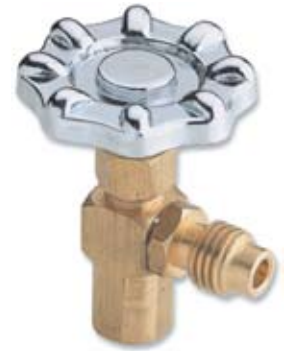
■ ■ CH-342 Can Tap Valve Forged brass body, strong and no leaking. Specially for R134A can 1/2" ACME female X 1/2" ACME male.
