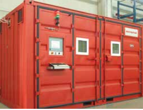
Proof pressure test stand able to pressurize hose assemblies up to 6.000 bar (87000 psi)
