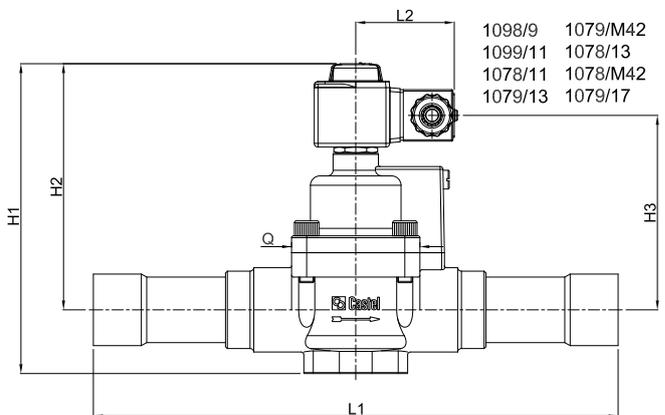
TABLE 3: Dimensions and weights of NC valves with 9300 coils (1)
