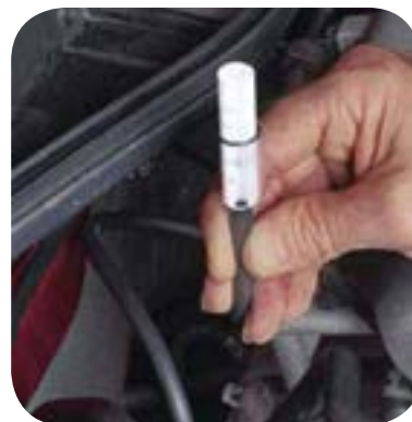
Flow meter quickly indicates presence of sealant
